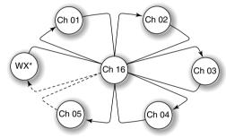
\*For USA, EXP, CHN and AUS versions. When the Weather Alert function is activated, the previously selected weather channel is also scaned.
