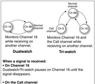
Tri-watch switches to Dualwatch until the signal on the Call channel disappears.
