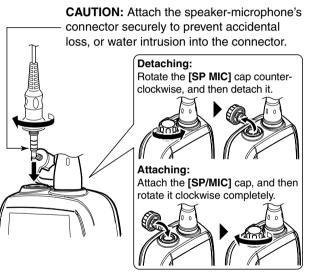
**IMPORTANT: KEEP** the transceiver's **[SP/MIC]** cap attached when the speaker-microphone is not used. If the cover is not attached, water will get into the transceiver. Moreover, the terminals (pins) will become rusty, or the transceiver will function abnormally if the connector gets wet.
