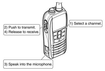
**IMPORTANT:** To maximize the readability of your transmitted signal, pause for a second after pushing **[PTT]**, hold the microphone 5 to 10 cm (2 to 4 inches) from your mouth and speak at a normal voice level.
